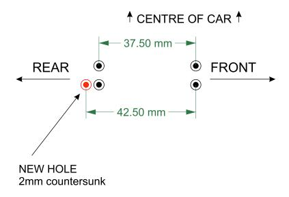
Place this template on the underside of the chassis and line up the 4 blck holes with the existing holes in your chassis. Drill a 2mm hole in the chassis through the red hole in the template and countersink to suit.
